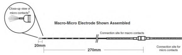
Note #3: Micro wires extend 20 mm past the tip; trim to the desired length before use.
