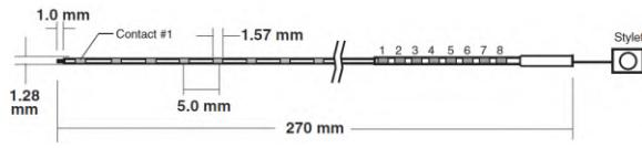
**Figure 2 – Wire Bundle Depth Electrode**
